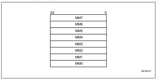
Although the MMX registers are defined in the Intel architecture as separate registers, they are aliased to the registers in the FPU data register stack (R0 through R7). (See Chapter 10 in the *Intel Architecture Software Developer's Manual*, Volume 3, for a more detailed discussion of MMX technology register aliasing.)
